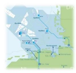
Wirescan Digital (WD) includes the whole TenneT Offshore GmbH portfolio of grid cables linking offshore wind farms in the North Sea to the onshore extra-high voltage grid. WD includes a large historical database. Cables are tested regularly when de-energized; data analysed where analysis is done automatically with comparison, trending and aging evaluation. Results and data are available to multiple stakeholders online in a meta-contextual map visualization
