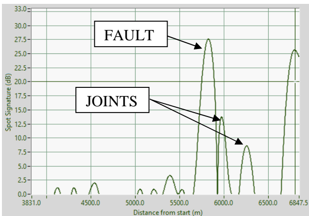
FIGURE 8 Fault localization close to a joint
