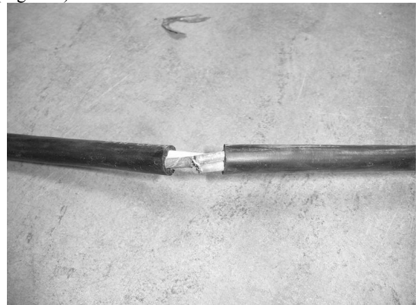
FIGURE 8 INSULATION CUT ON XLPE SAMPLE
